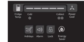
**Lock blocks the external control and prevents any accidental change in the configuration. Activate/deactivate it pressing the button for three seconds.**
