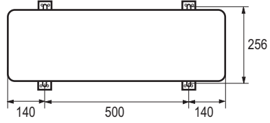
Outdoor unit floor fixing dimensions. Units in mm
