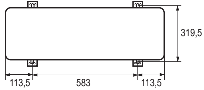
Outdoor unit floor fixing dimensions. Units in mm
