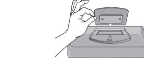
4 Close the lid, put the tank back in its place and push it to the very end. The water will be poured into the ice tray.
