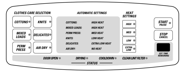
**NOTE**: Any time you make a selection that is incompatible with the chosen dry cycle, the dryer will beep twice.
